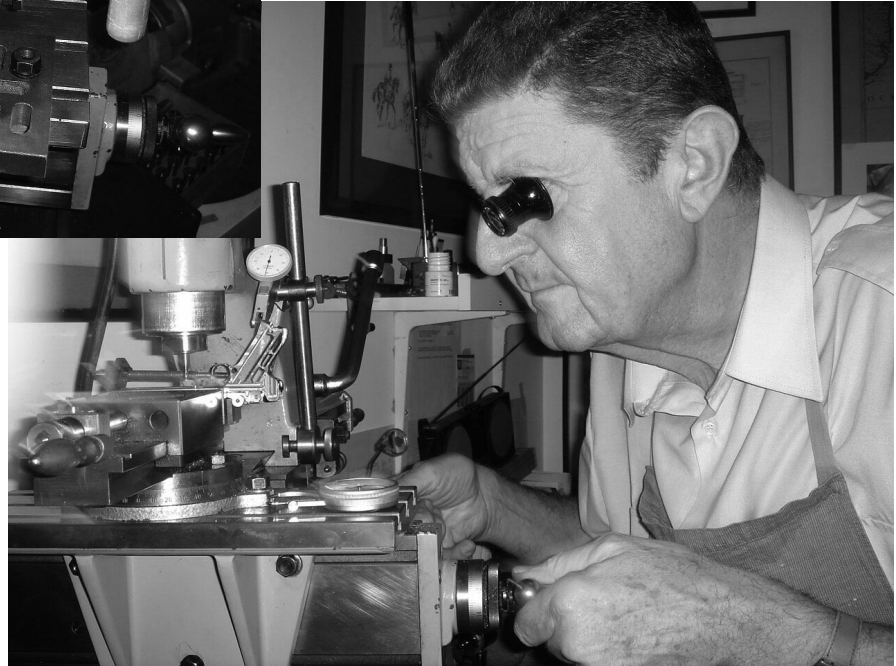
Below: Michel performing a precision milling operation on the main frame.
